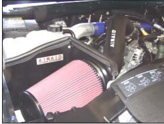
14. Install the Airaid Premium Filter (#1) onto the filter adapter, and tighten the hose clamp. Install the weather strip (#8) onto the Airaid Cool Air Dam. Reconnect the M.A.F. sensor wiring harness. ( Note: Start from one corner and work your way around to insure proper alignment of the weather strip. )
