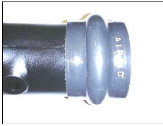
11. Install the urethane hump hose (#6) and two #72 hose clamps (#17) onto the large end of the Airaid intake tube. ( Note: Leave hose clamps loose until final assembly. )
