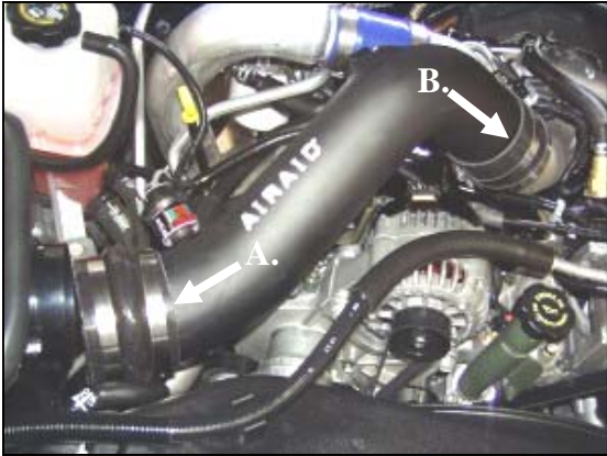
13. A.) Install the hump hose end of the Airaid intake tube assembly onto the filter adapter first. B.) Slip the coupler end of the tube over the factory turbocharger inlet. Adjust for fit, and tighten the hose clamps. ( Note: There should be a gap between the Airaid intake tube and the air filter adapter. )
