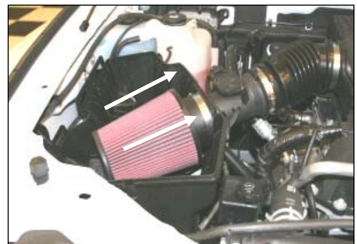
6. Make sure the filter and the hose clamp are pushed close to the factory airbox wall, and tighten the hose clamp as shown. Do Not over tighten.
