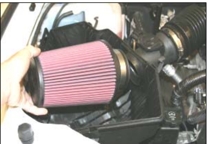
5. Install the Airaid Premium Filter (#1) on the factory intake tube.
