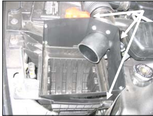
11. Install the Quick Fit Panels onto the top of the factory air box base. Relatch the factory clips onto the tabs on the Quick Fit Panels.
