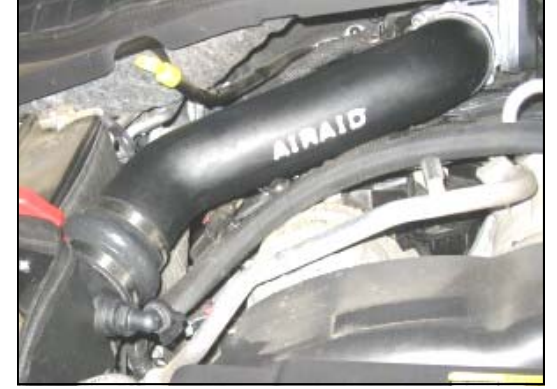
15. Install the Airaid Intake Tube assembly onto the engine with the hump hose end towards the air filter adapter. Adjust the assembly for fit and then tighten the four hose clamps.
