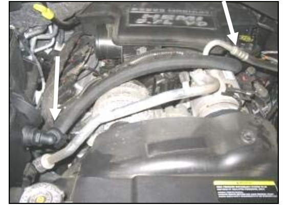
12. Remove the factory breather hose. Connect one end of the 3/4" x 25" hose (#5) to the nylon fitting and the other to the oil fill nipple as shown. Secure each end using one #24 Speed Clamp (#16). Adjust the nylon fitting downward to clear the Airaid Intake Tube assembly.
