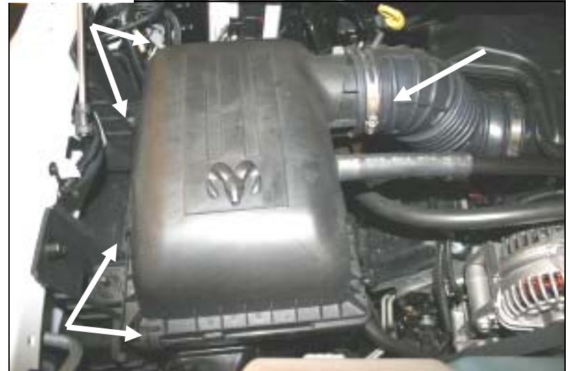
2. Unlatch 4 clips that hold down the factory airbox lid. Loosen the hose clamp on the factory intake tube where it connects to the airbox lid, then remove the lid.
